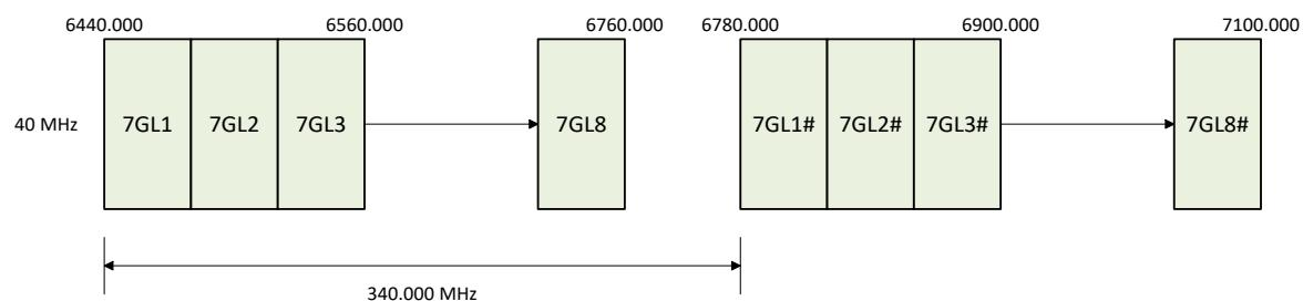
This band is designated for use by digital high capacity fixed point-to-point links.
