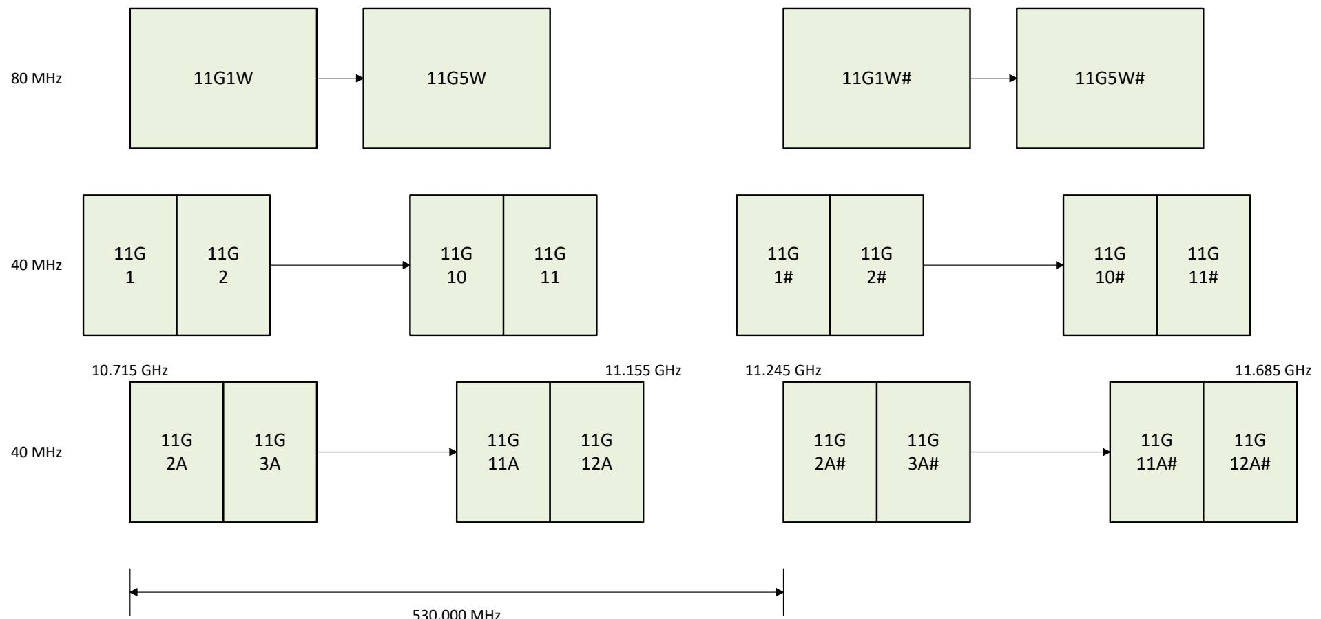
Note that the two groups of 40 MHz channels are interleaved.
