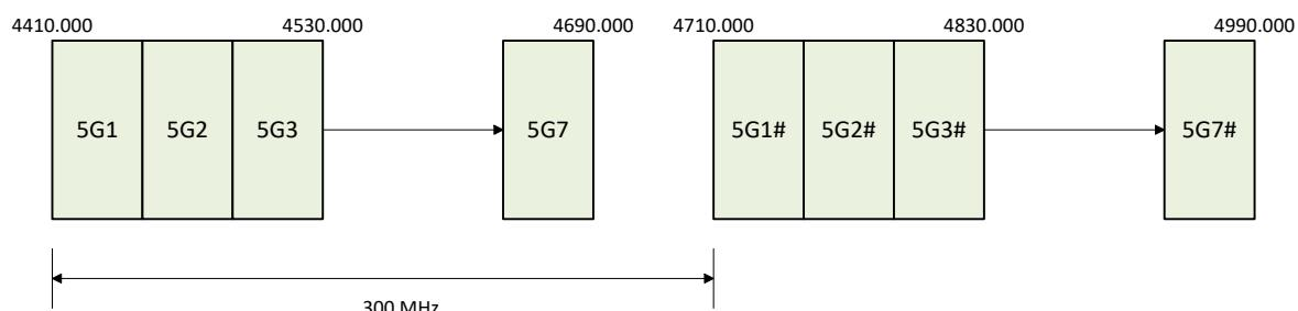
This band is designated for use by digital high capacity fixed point-to-point links. Proposed links need to be coordinated with satellite Earth stations operating in this band. See Radio Licence Certification Rules (PIB 38) and Radio Licence Policy Rules (PIB 58) for further details.
