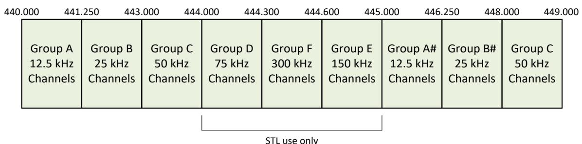
The JL band is restricted for digital services only with a minimum spectral efficiency of 2 bits per second per Hertz. The 75, 150, and 300 kHz channels are for Studio to Transmitter Linking (STL) only. These (STL only) channels are not subject to digital criteria.
