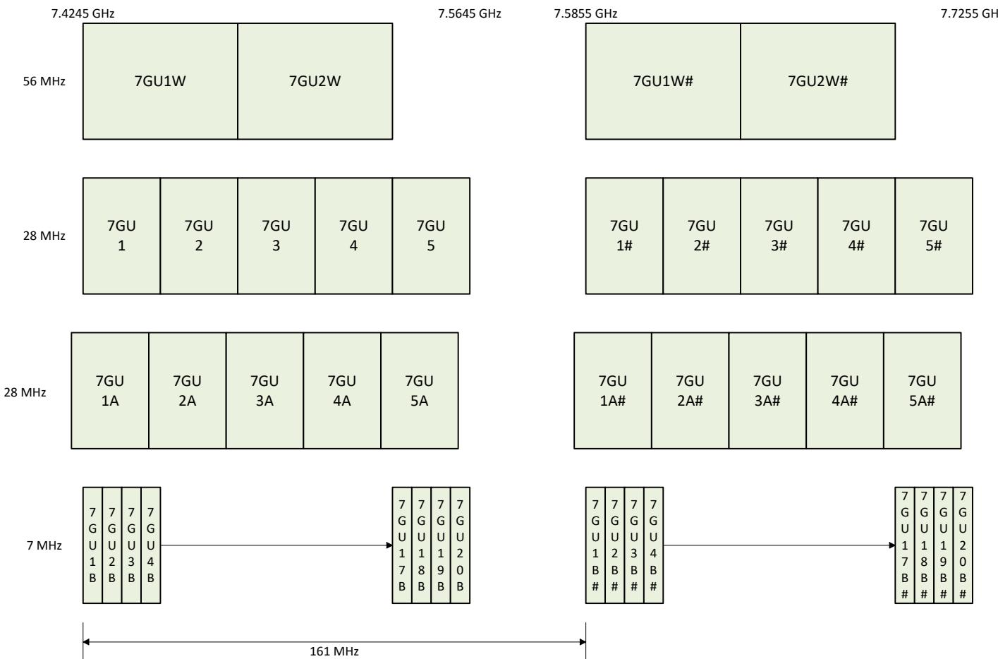
Note: 56 MHz channels are restricted for DMR with a minimum spectral efficiency of 4 bits per second per Hertz. See Radio Licence Certification Rules (PIB 38). The following 28 MHz (7GUA) channel plan is not the preferred plan and is recommended only for legacy services and equipment.
