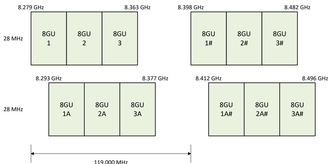
The 8GU<sub>n</sub> channels are legacy channels and consequently unavailable for new services. The two groups of channels are interleaved.
