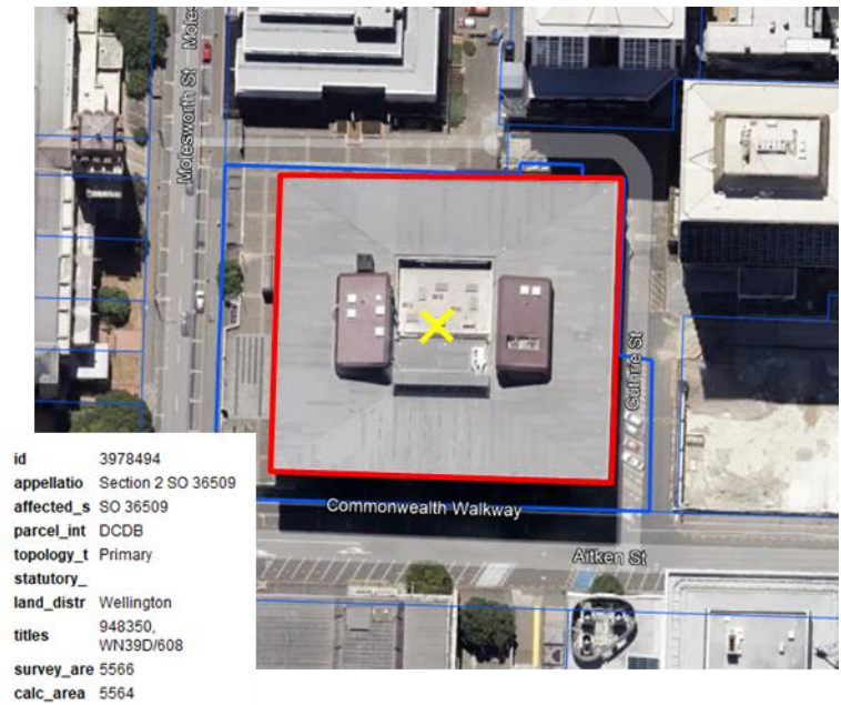
Figure 10: Sample indoor licence area for building in relevant land parcel (Blue), with BS Licence location at building centre (Yellow) with licence area polygon matching building footprint (Red)
