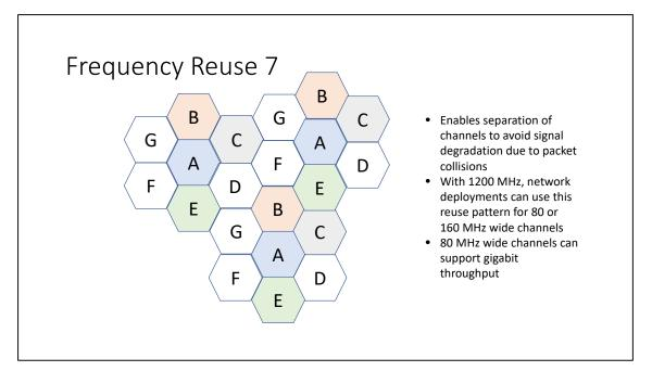
The frequency reuse 7 methodology minimizes packet collisions that degrade throughput by keeping "like" channels separated. With the full 1200 MHz authorized, government and enterprise deployments have access to up to fourteen 80 MHz wide channels and up to seven 160 MHz wide channels. This is important because the 80 MHz wide channels are what can deliver gigabit throughput, which will be a necessity soon and is desirable now.
