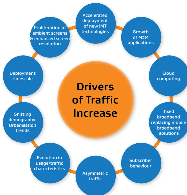
▶ Figure 3: Drivers of mobile traffic increase 2020-2030 (source: ITU Report M.2370-0 (07/2015))
