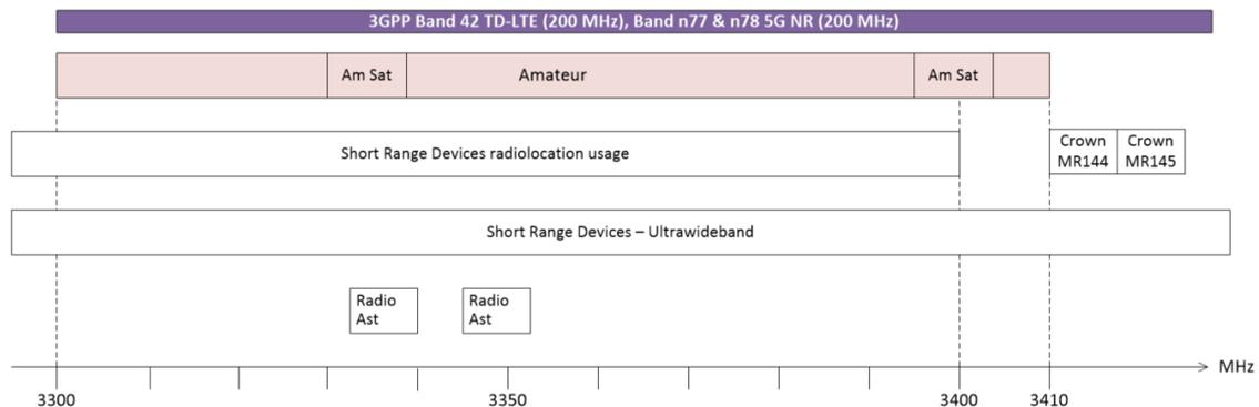
**Figure 1 Current Spectrum use between 3.30 and 3.41 GHz**
