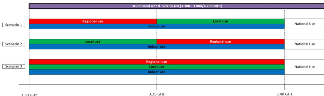
**Figure 2 Deployment scenarios and options for the 3.3 GHz band**
