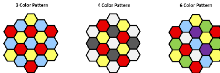
Figure 6: Examples of Satellite Spot Beams and Spectrum Reuse
